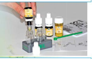
Move the comparator block with the two test containers backwards and forwards on the colour chart with the notch pointing to the values, until the colour of the sample treated with reagent matches the colour under the blank sample as closely as possible.
